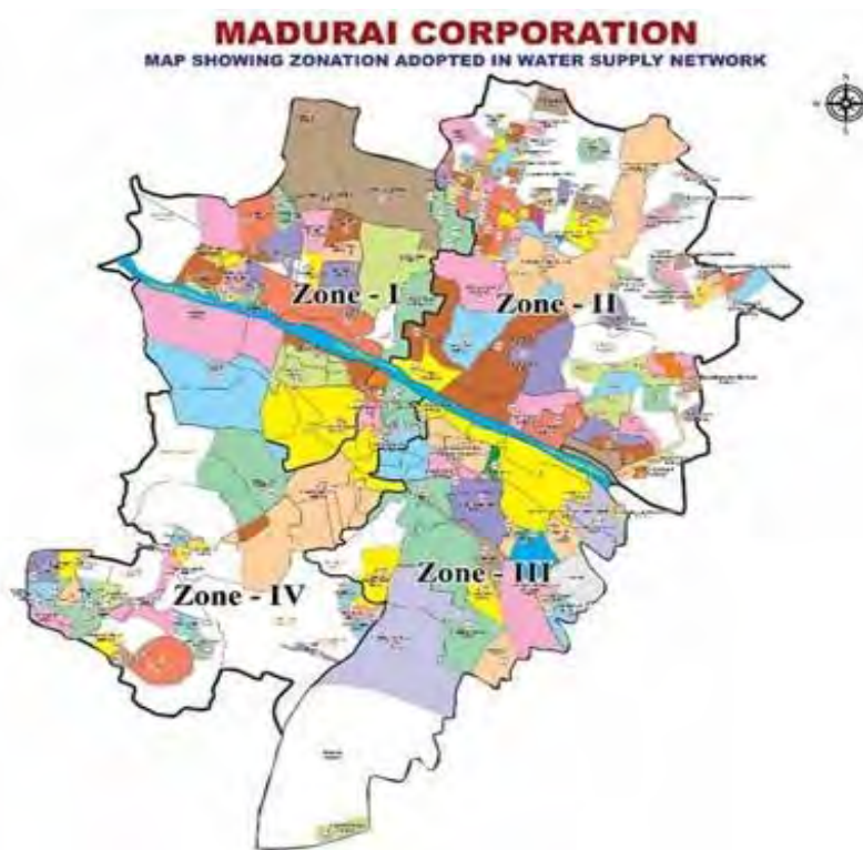
Figure 2: Water Supply Zones of Core Madurai
